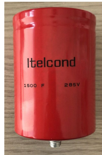
Figure 9. Final SC-GN3 "zero prototype" of wound supercapacitor with 1500F / 2.85V active element inside
